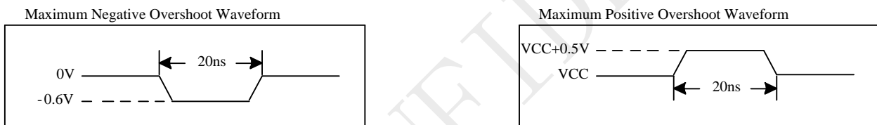
Figure 5-1 Maximum Overshoot Waveform
